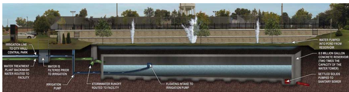
Figure 7. Example of stormwater collection and reuse project in St. Anthony, Minnesota. ( http://www.wsbeng.com/Services/ProjectPages/sustain_Reuse.html )
