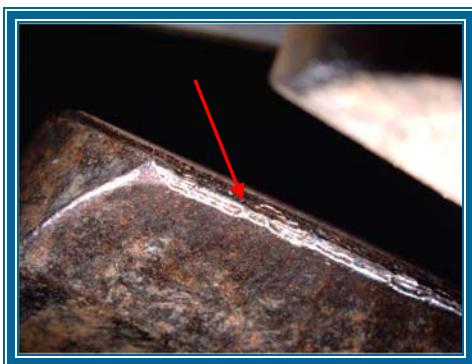
Copper on the blades of the wire cutters
