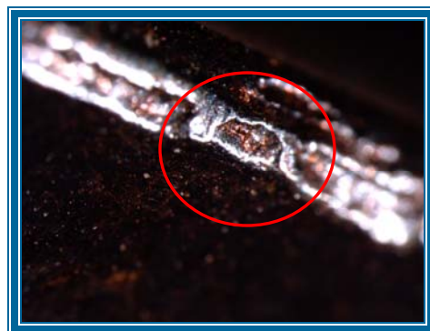
Copper on the blades of the wire cutters
