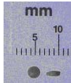
Figure 6: Front and side view of microdots.
