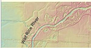
1-meter resolution data with 1/2 foot vertical accuracy
