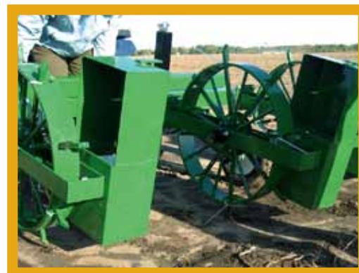
Figure 7: Collecting soils samples with a mechanical sampler
