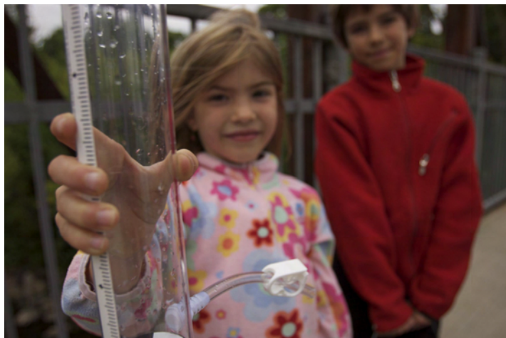
Figure 4: CSMP volunteers measure stream transparency using a transparency tube.
