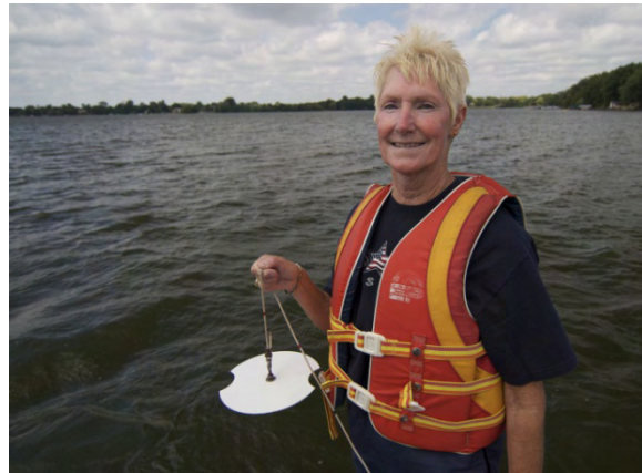
Figure 2: CLMP volunteers use Secchi disks to monitor lake transparency.
