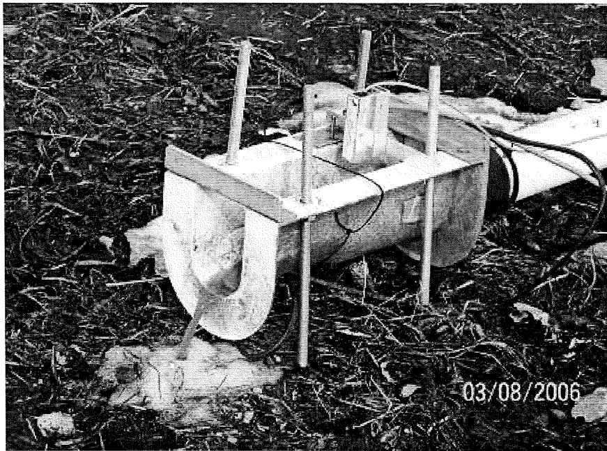
Figure 37: Biofilter discharge flume including flow sensors
