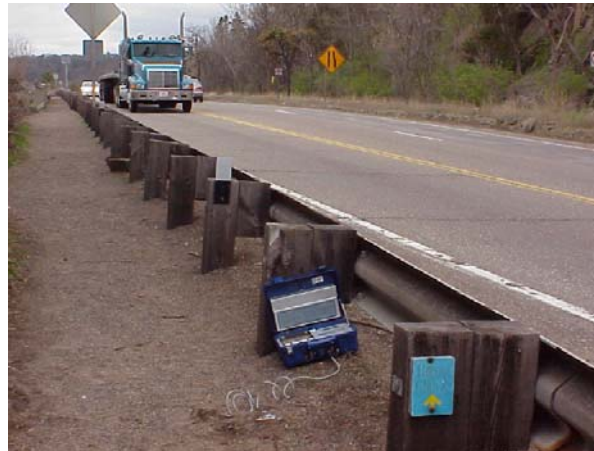
Mn/DOT equipment used to monitor traffic vibration and impact on surrounding land. Photo by Carmelita Nelson, DNR.
