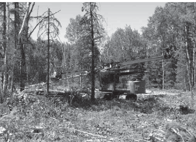
▲ Harvesting methods are one important factor considered when developing a silvicultural prescription. Advances in technology have changed forest harvesting methods, such as the use of this stroke delimber to remove branches from harvested trees, a job which used to be conducted by loggers with chainsaws. Photo: MFRC Staff.
