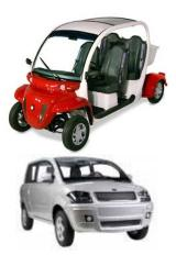
The electric vehicles are rechargeable through the electrical grid and have a range of between 30 to 75 miles before needing to recharge. Models come in styles ranging from two-seaters to small-scale trucks, normally weighing 1,000 to around 1,500 pounds. They have primarily been produced for niche uses such as military bases and retirement communities, but their use is widening. Demand also grew out of combined use on golf courses and adjacent streets. The largest U.S. market is in California.
