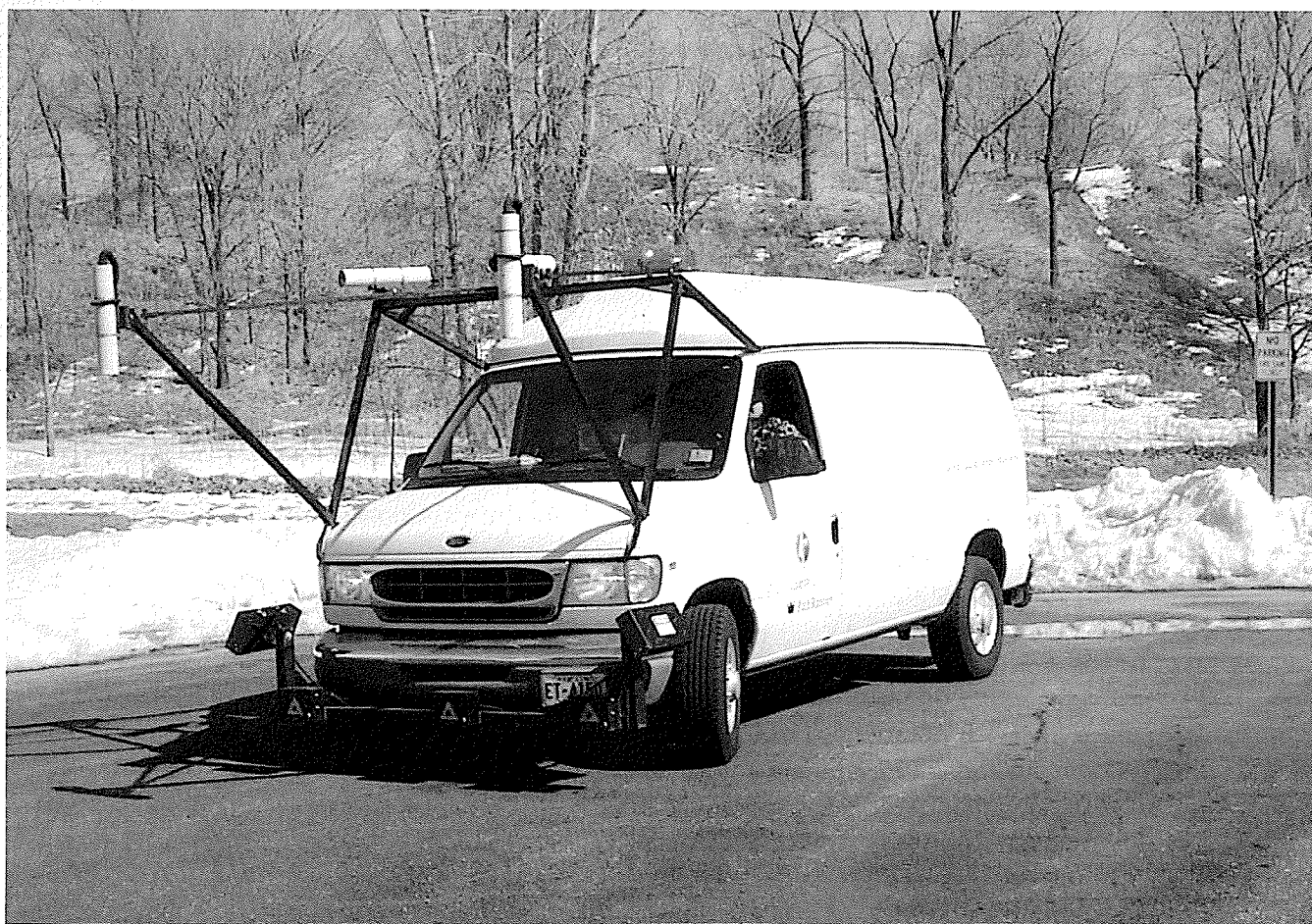
Figure 3-1 Pavement Management Van
