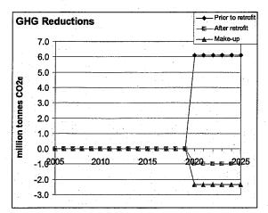
Figure G-23. GHG emission reductions from retrofitting existing pulverized coal stations with CCS
