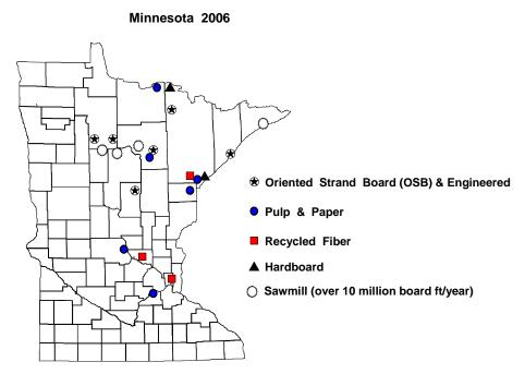
Location of mills is an important factor in determining markets for wood. The map above shows the OSB, pulp & paper, recycled fiber, hardboard, sheathing and large sawmills in Minnesota. These mills utilize various species of wood material, with aspen pulpwood being by far the largest component.
