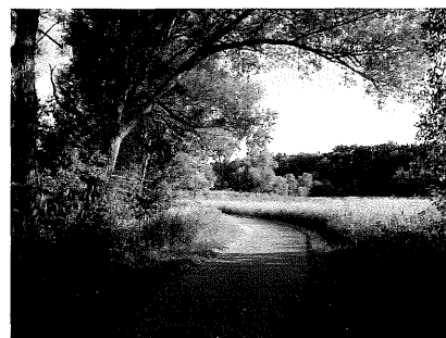
This is a typical city or county trail through an established greenway corridor. A 10-foot width is optimal on most trails, but 12-foot widths are also used in very heavy use areas.
