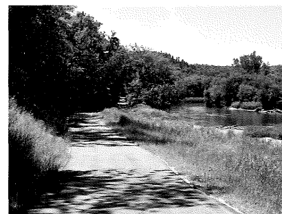
This is a typical regional or state trail through an established rails-to-trails greenway corridor. A 10-foot width is the minimum recommended.
