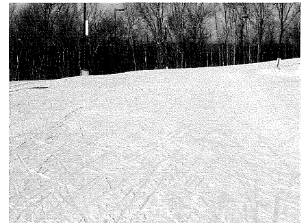
Skate style - double width/one or two directions. This trail type is occasionally used in a county, regional, or state park where use pressures are high and/or where separation of skiing styles is preferred. They are not as common as combination trails due to increased kilometers needed to accommodate separated uses, and the more time needed for grooming. Total width is 14 to 16 feet.
