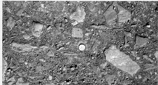
This well-graded aggregate tread is very stable with the right subgrade soil conditions. In other soils, this may not have enough variety in size and shape of rocks and soil particles to be stable. Site evaluation is critical to determining the type of aggregate needed to create a sustainable trail.
