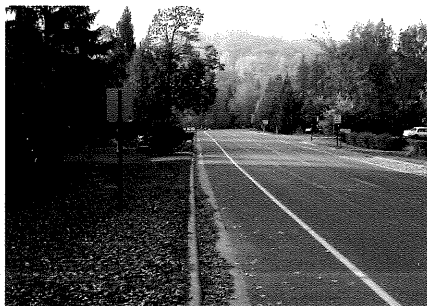
Bike lane with curb and no parking. 5 feet wide from face of curb, with a 4 feet desirable from left of the gutter edge. On one-way streets, the bike lane can be on the right or left side of the road, depending on parking and other site characteristics.
