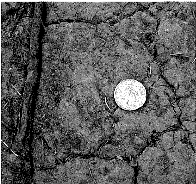
A slightly gravelly loam has clay, silt, sand and small rock particles. It is firm when dry and makes a relatively durable tread surface. Shrinkage cracks indicate the presence of expansive clays, which are excellent binders but very slippery when wet.
