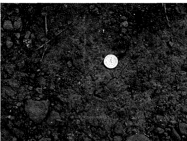
Loam with some rocky material on the Superior Hiking Trail makes a durable tread.
