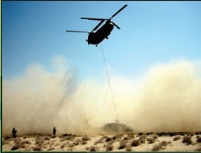
◀ A Minnesota National Guard CH-47 Chinook helicopter sling-loads a UH-60 Blackhawk helicopter in March preparation for movement in southern Iraq.
