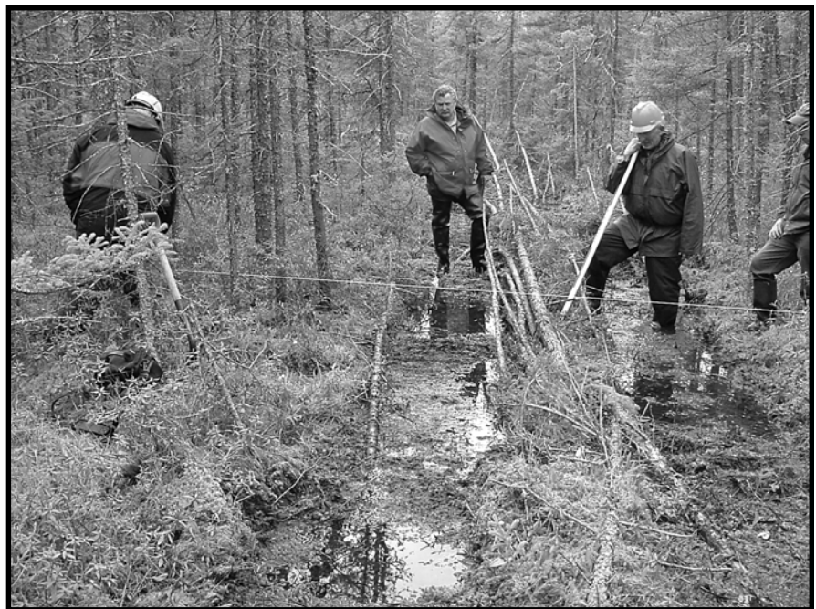
A monitoring team uses string levels to evaluate depth of rutting in a black spruce stand. Photo by Mike Phillips, MFRC
