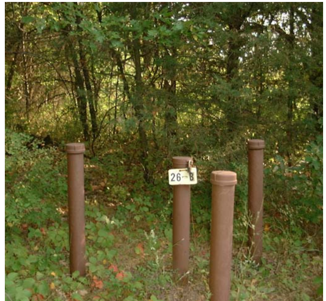
Photo 6: Anoka-Ramsey Landfill monitoring well
