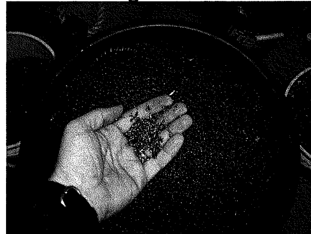
Iron Fillings for Scrubber
