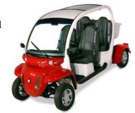
NEVs have primarily been produced for niche uses such as military bases and retirement communities, but their use is widening. The largest U.S. market is in California. The vehicles are rechargeable through the electrical grid and have a range of between 30 to 75 miles before needing to recharge. Models come in styles ranging from two-seaters to small-scale trucks, weighing 1,000 to around 1,500 pounds. Prices start at about \$8,000.
