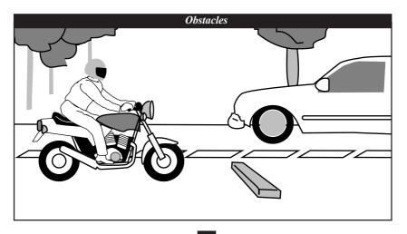
If you ride over an object on the street, pull off the road and check your tires and rims for damage before riding any farther.
