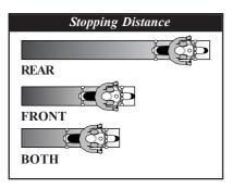
Always use both brakes at the same time to stop. The front brake can provide 70% or more of the potential stopping power.
