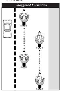
A third rider maintains in the left position, two seconds behind the first rider. The fourth rider would keep a two-second distance behind the second rider. This formation keeps the group close and permits each rider a safe distance from others ahead, behind and to the sides.
