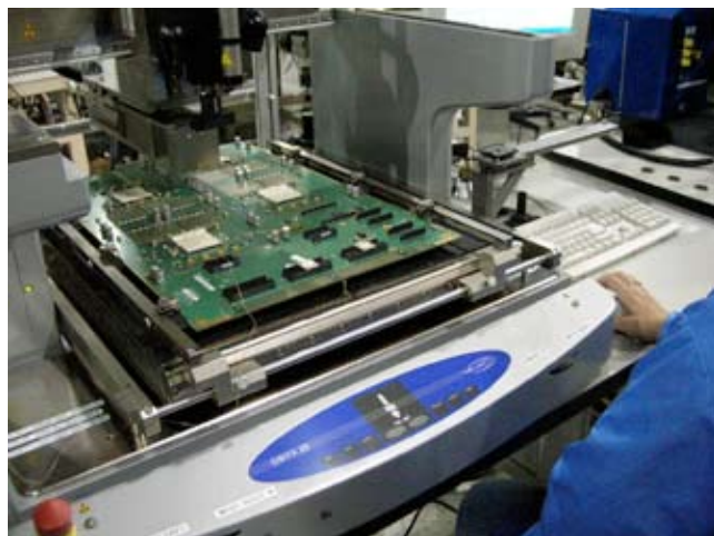
Rework equipment used as part of the non-lead solder assembly process at Benchmark Electronics (Winona).
