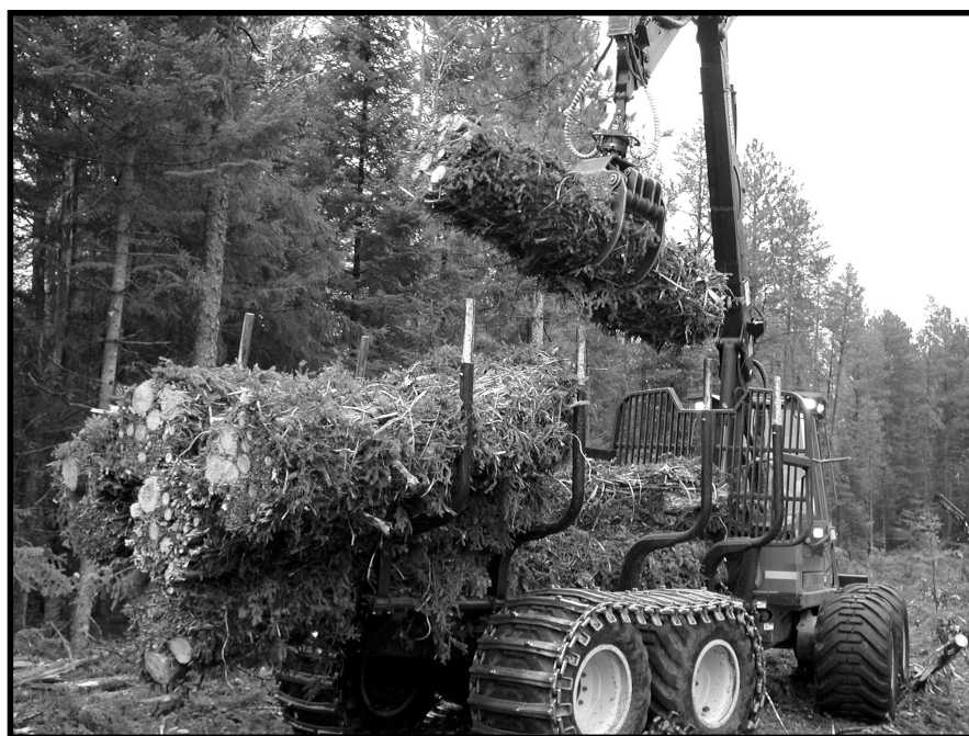
Biomass harvesting includes collecting bundles of slash for use in generating energy. Photo by Dave Chura
