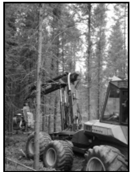
Timber harvesting is often done via expensive mechanized forestry harvesters like this one. Trees are delimbed and cut to length directly at the stump area. Photo by Dave Chura
