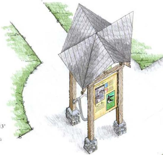
AXONOMETRIC DRAWING OF KIOSK WITH BIKE RACK AND INTERPRETIVE PANELS
