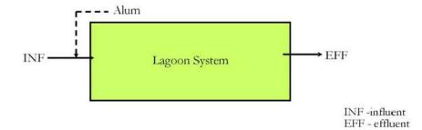
Figure 4.5 - Chemical Precipitation is the Phosphorus Removal Alternative for Lagoons
