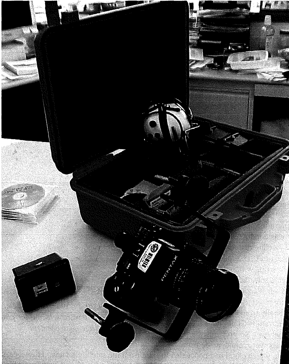
Figure 5: Resource Assessment photographers used Pentax 645-format cameras (shown above with aerial mount) and Kodak Portra 400VC color-negative film. The 41x56mm format size captures more detail than 35mm photography at equivalent scales. Photos were produced as nominal 1:6000 scale prints and scanned at 300ppi for interpretation.
