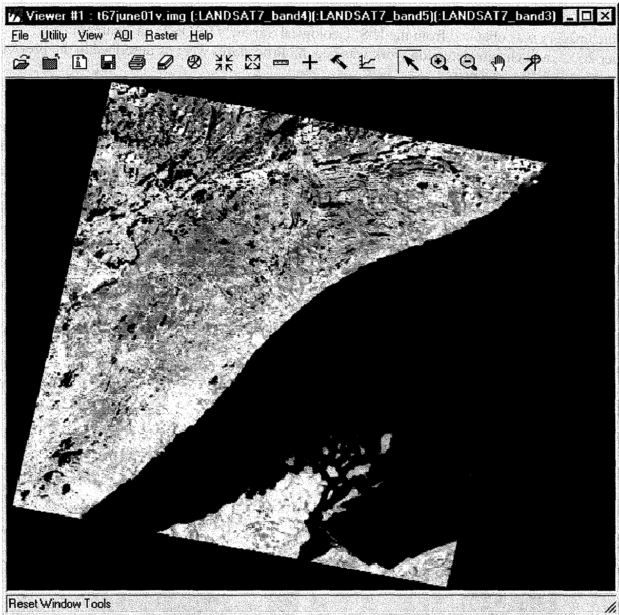
Figure 2: A single Landsat 7 ETM multispectral image covers 7.7 million acres. Each individual picture element covers a 100-foot square on the ground, and contains information from six bands in the visible, near-infrared and mid-infrared portions of the electromagnetic spectrum. Current purchase price is only $600.
