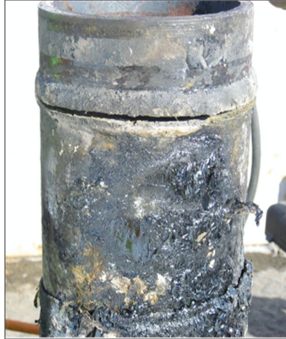
Left: Crookston Campus - ruptured natural gas pipe
