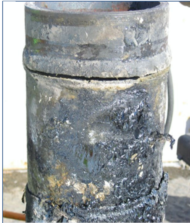
Left: Morris Campus - ruptured natural gas pipe
