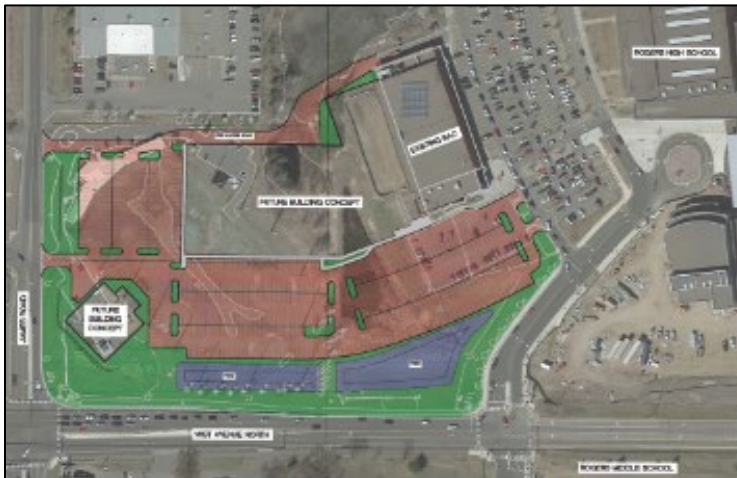
Site Improvements For Future Recreational Facilities: Includes stormwater, parking and site preparation
