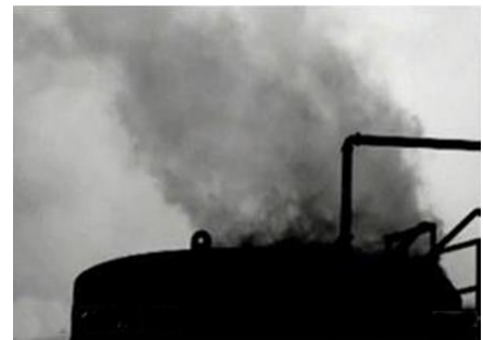
To the naked eye, no emissions are visible. With infrared imaging, methane emissions
