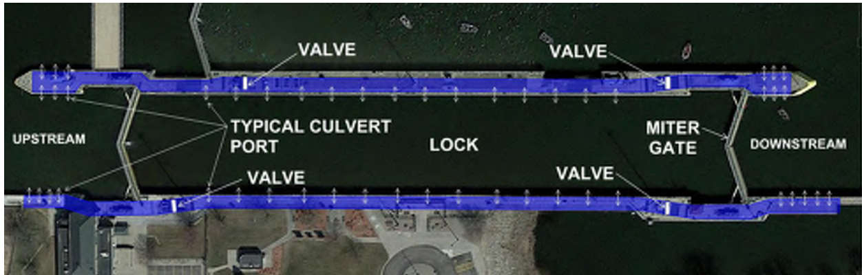
Figure 2-2 Lock layout and discharge ports
