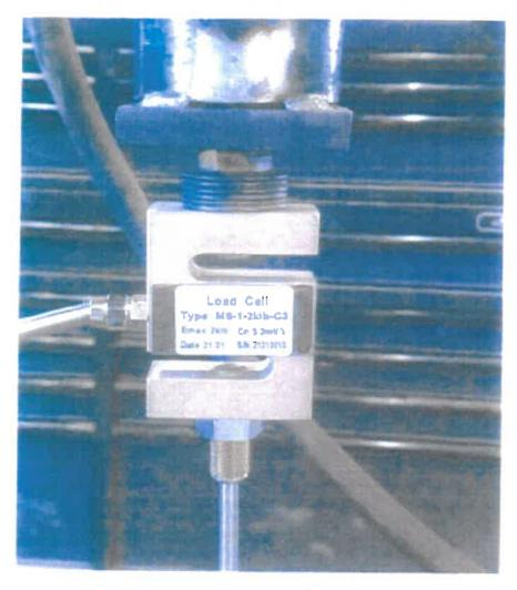
We tested the accuracy of the load cell against the accuracy of a bench scale at very light pressures, as we did not want to dent the surface of the bench scale with the tiny probe so we kept the pressures light. The load cell would be more accurate if we took it up to somewhere mid-range, but our purpose was to insure it was working properly. The accuracy is displayed below. At this very light weight the accuracy is 40% which is very acceptable.
