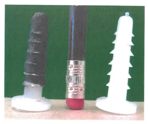
This picture shows the mastic on the plug to provide additional sealing in addition to the plug. It should be noted that the covers of all the tanks set in place via gravity with only a mastic seal and it functions well in the field.
