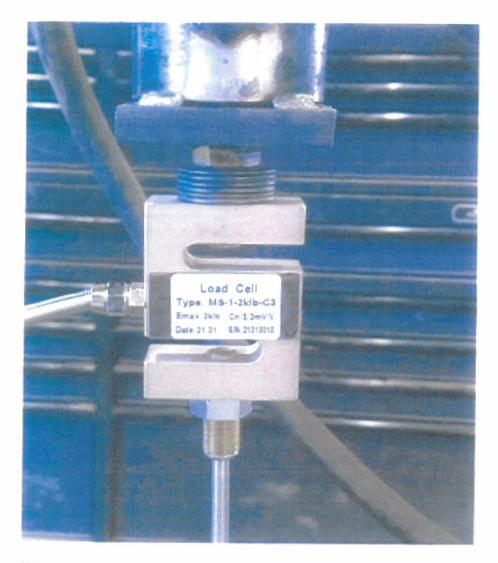
We tested the accuracy of the load cell against the accuracy of a bench scale at very light pressures, as we did not want to dent the surface of the bench scale with the tiny probe so we kept the pressures light. The load cell would be more accurate if we took it up to somewhere mid-range, but our purpose was to insure it was working properly. The accuracy is displayed below. At this very light weight the accuracy is 9% which is very acceptable.
