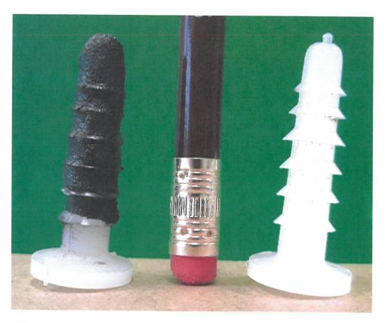
This picture shows the mastic on the plug to provide additional sealing in addition to the plug. It should be noted that the covers of all the tanks set in place via gravity with only a mastic seal and it functions well in the field.
