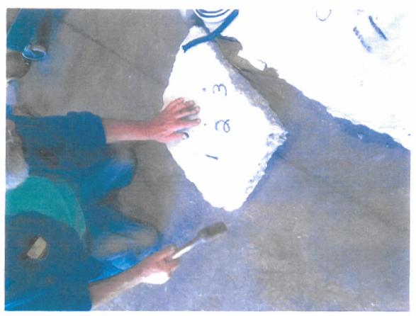
The pieces that we used for the test were from the 3" thick walls of a scrap tank that is the same model wherein some of the drain holes were drilled. We drilled a sample set of 12 holes, installed the plugs with and without the aid of mastic sealer (mastic was installed in all of the tanks that were installed in the field). It should be noted that the plugs fit so tightly in the holes that a hammer is required to pound them in as they will not push in by hand. See the picture above.
