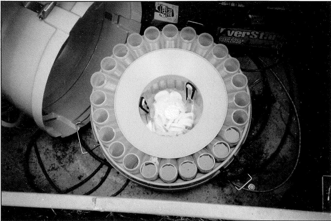
Inside an ISCO sampler - sampling bottles.
