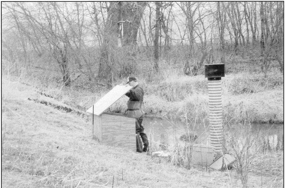
An ISCO sampler is housed in a locked wooden or metal box to prevent damage from the elements and the curious.
