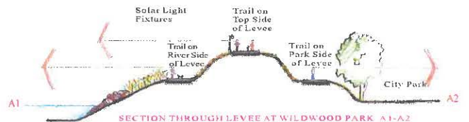
SECTION THROUGH LEVEE AT WILDWOOD PARK A1-A2
