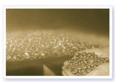
The successful production of iron nuggets with a 96% metallic iron content expands the taconite industry's customer base to include electric arc furnace operators and foundries.
