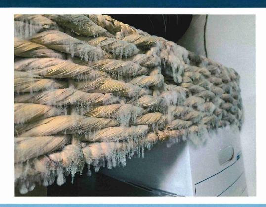
Mold growth in a basement area converted and used as staff office space with inadequate ventilation and high humidity levels
