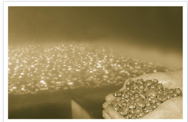
*The successful production of iron nuggets with a 96% metallic iron content expands the taconite industry's customer base to include electric arc furnace operators and foundries.*
