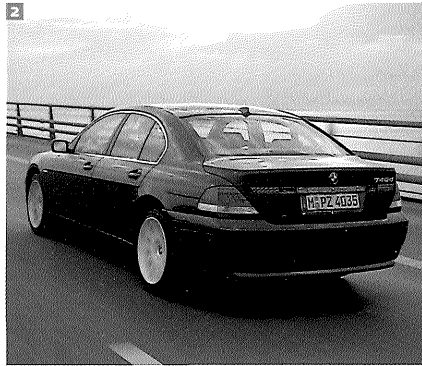
1 In Europe, the 2003 BMW 530d gets 30.2 MPG, versus 23.8 MPG for its gasoline counterpart. 2 The 2003 BMW 740d sedan gets 28.9 MPG, compared to 24.4 MPG for the gasoline version.
