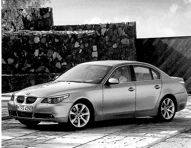
1 In Europe, the 2003 BMW 530d gets 30.2 MPG, versus 23.8 MPG for its gasoline counterpart. 2 The 2003 BMW 740d sedan gets 28.9 MPG, compared to 24.4 MPG for the gasoline version.
