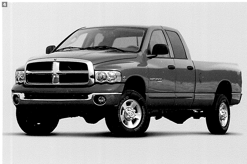
4 The diesel electric hybrid Dodge Ram heavy-duty pickup has an integrated starter-generator powertrain that produces up to 10 percent better fuel efficiency and enhanced performance on the road. Off the road, the powertrain converts to a clean generator to provide electric power in remote sites.
